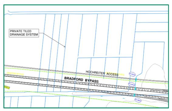
Figure 1: Private Drainage System along Bradford Bypass
