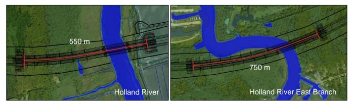
Based on these parameters, the minimum bridge span for the Holland River and Holland River East Branch were selected at 550 m and 750 m respectively, as shown in **Figure 10**.
