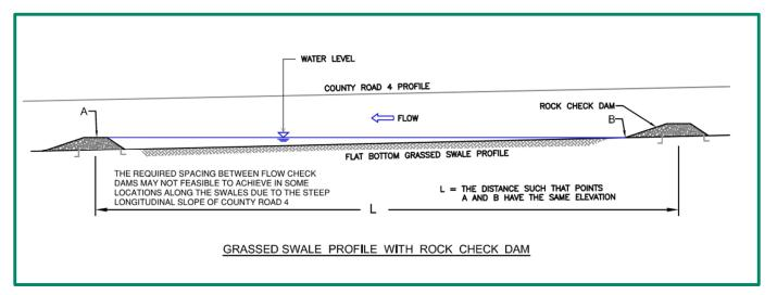
Figure 14: Conceptual Locations of Flow Check Dams Along Flat Bottom Grassed Swale
