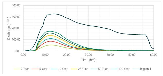
Figure 2: Flow Hydrographs at the Holland River Highway Crossing
