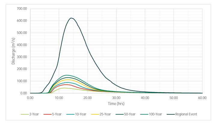
Figure 3: Flow Hydrographs at the Holland River East Branch Highway Crossing
