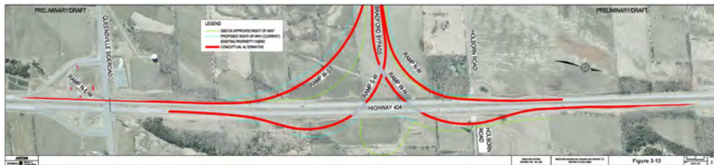
Figure 3-13: Extend Two Lane Ramp from Bradford Bypass Eastbound Ramp and Close Queensville Sideroad Off-Ramp (Alternative 2)
