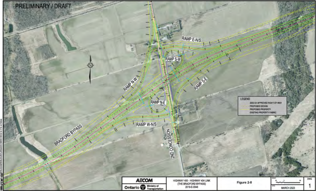
Figure 4-8: Recommended Plan for the 2 nd Concession Road Interchange
