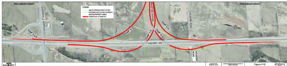
Figure 3-12: Extend Two Lane Ramp from Bradford Bypass Eastbound Ramp to Queensville Sideroad Ramp (Alternative 1)
