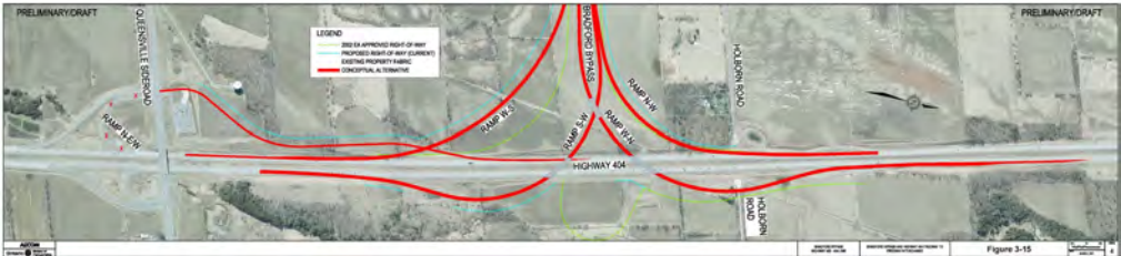
Figure 3-15: Basketweave Ramp Connection to Queensville Sideroad (Alternative 4)
