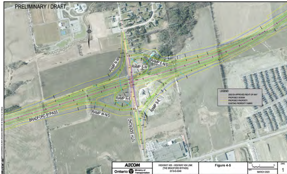
Figure 4-5: Recommended Plan for 10 th Sideroad Interchange
