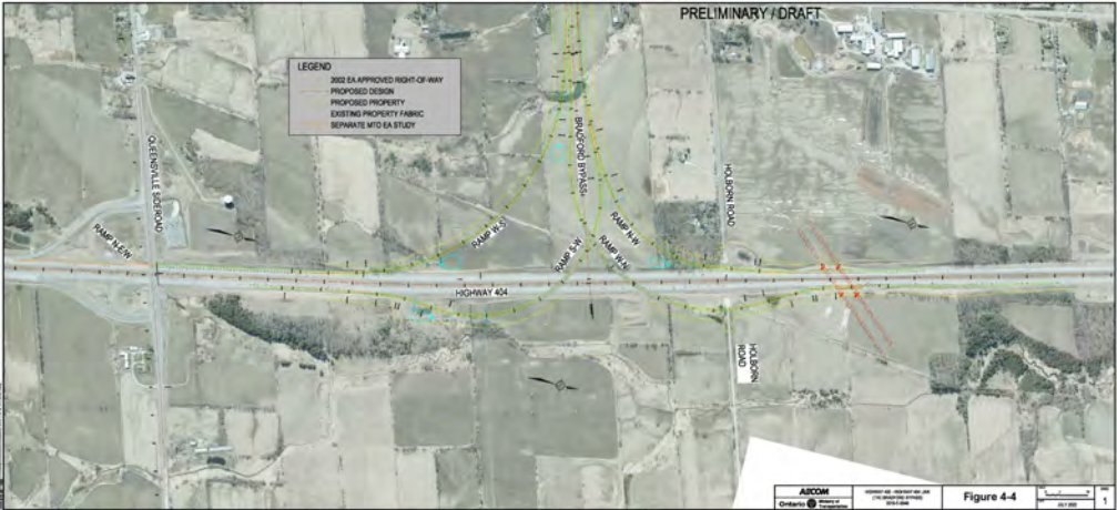
Figure 4-4: Recommended Plan for the Highway 404 Freeway-to-Freeway Interchange
