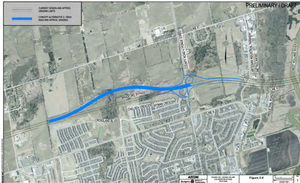
Figure 3-4: Alignment Shift with 1300 metre Radii Curves (Alternative 3)
