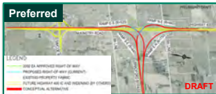
Alternative 3 – 525m Radius Bradford Bypass to 400 Southbound Ramp with Lanes to County Road 88
