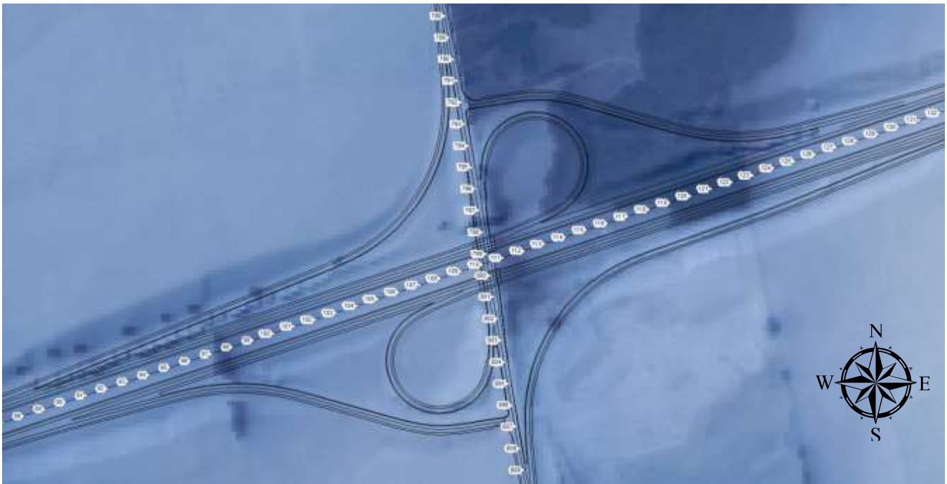
Figure 20 Example of Point of Interest (POI) distribution along the highway route and Interchange at 25m
